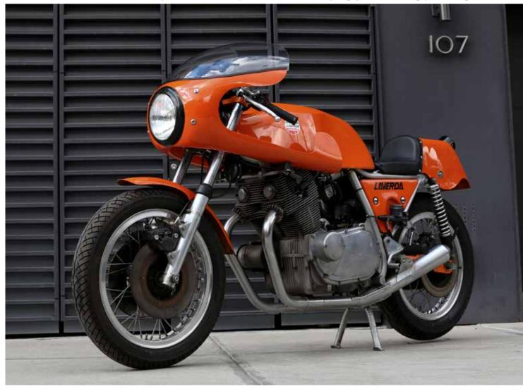
Two of the most significant updates for 1974 was the pair of Dell'Orto PHB 36 carburetors, without accelerator pumps, and twin-bleed Brembo F08 calipers with twin front discs, and a single rear disc on an Elektron hub. A racing two-into-one megaphone (as on this example) accentuated the lean race replica profile, and the claimed power for the 1974 750 SFC was 75 horsepower at 7,500 rpm. The right-side gear shift remained as did Borrani rims and Ceriani suspension front and back.
