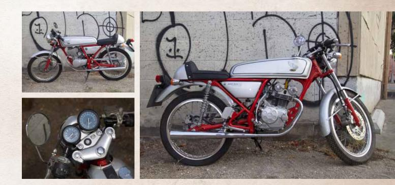
A modern homage to Honda's early Grand Prix road race bikes, two editions featuring race-only 50cc Honda motors with double-overhead camshafts and a 14,500-rpm redline is a masterpiece in miniature.
