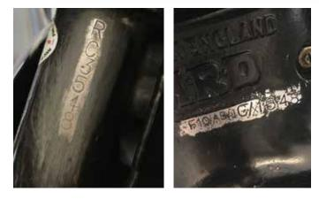
The Earls Court machine and 'RC3548' (the second Black Lightning) have rear frames with a single brake abutment; all subsequent examples have two abutments. In a letter on file, former Vincent employee Jack Lazenby, who was one of the select band charged with Black Lightning assembly, says that he cannot recall any numbers being stamped on the rear frame, and the one fitted to 'RC3548' is blank.
